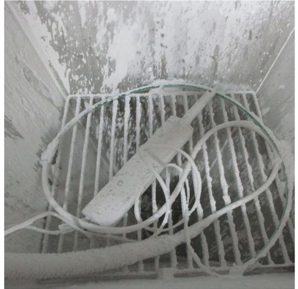
*The linear actuator during the IP65 (Degrees of protection) testing.*
